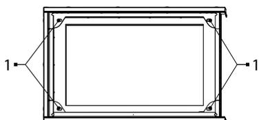
Fasten the cooler casing to the unit with screws.
