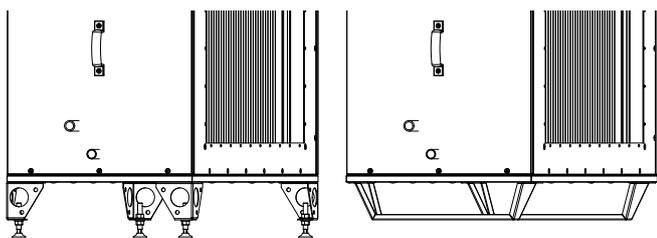
If the cooler is to be mounted on the floor, the feet must be screwed on.
