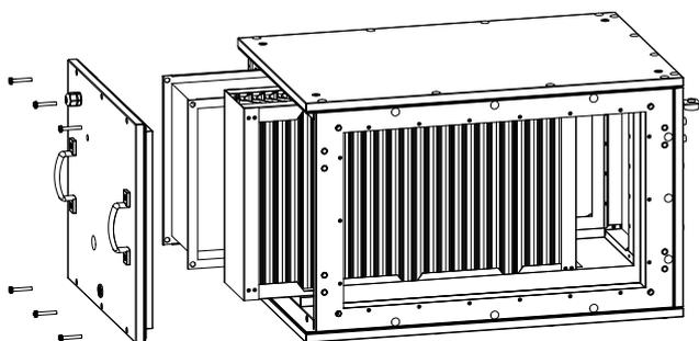
To connect the cooler to the unit, remove the front panel and remove the cooling unit and droplet separator.
