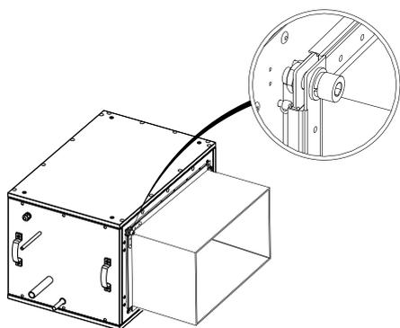
The cooler is connected to the air duct using a flange connection.
