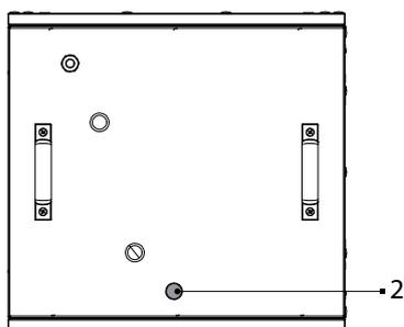
The DX coolers are equipped with a drain pan for condensate collection. The condensate is drained off via the drain pipe (2)
