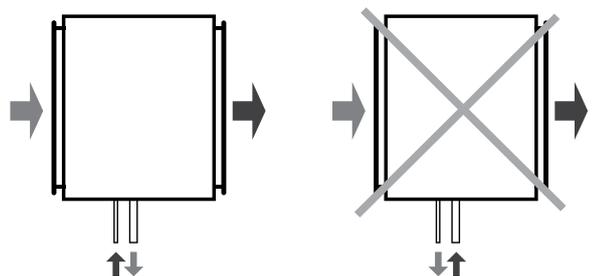
To attain the maximum capacity, the cooler must be connected on counter-flow basis.
