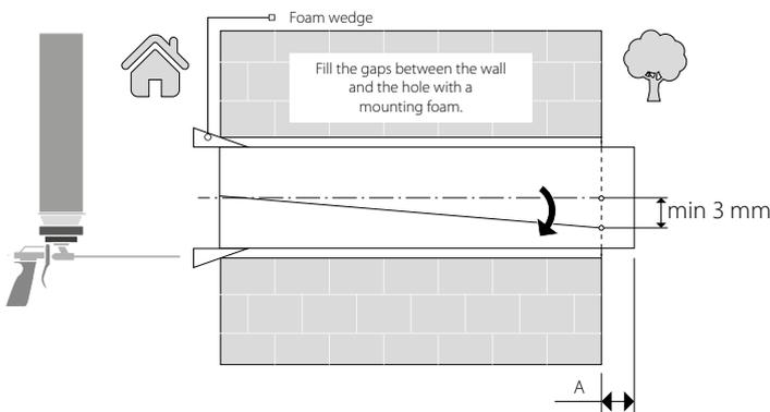
While mounting the air duct be sure to provide the minimum slope of 3 mm downwards from outside.
