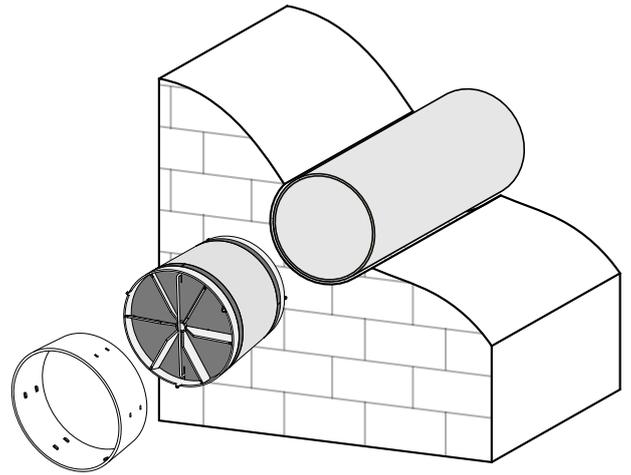
4. Use a screwdriver to unscrew the self-tapping screw from the casing and remove the front part of the indoor unit.
