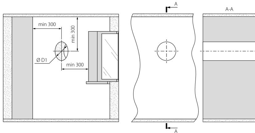
2. Install the air duct into the hole so that its cuts are aligned with the outside and inside surface of the wall. For ease of installation use the foam wedges included in the delivery.
