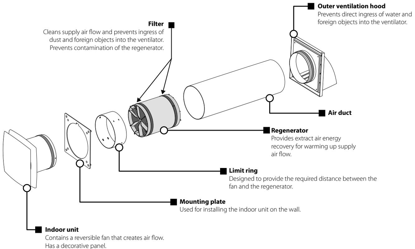
The ventilator operates in two cycles, 60 seconds each.
