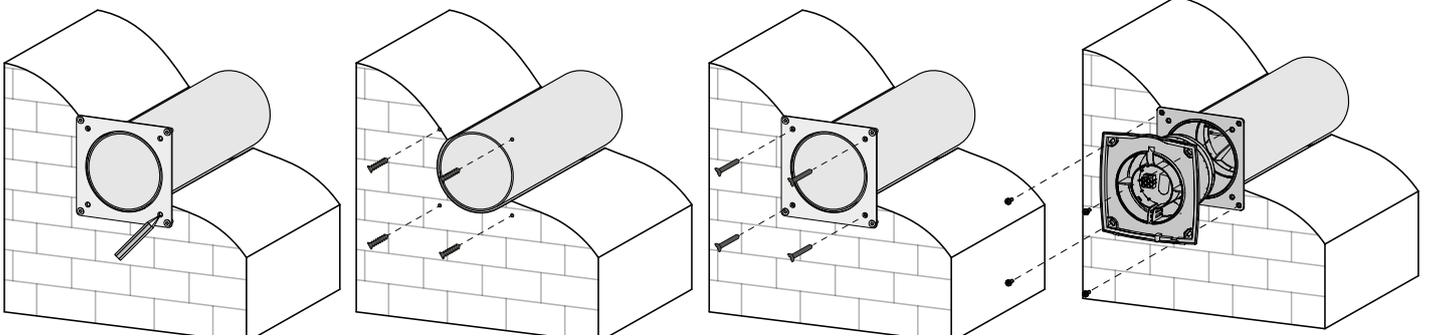
6. Install the front part of the indoor unit to its original position and fix it with a screw using a screwdriver.
