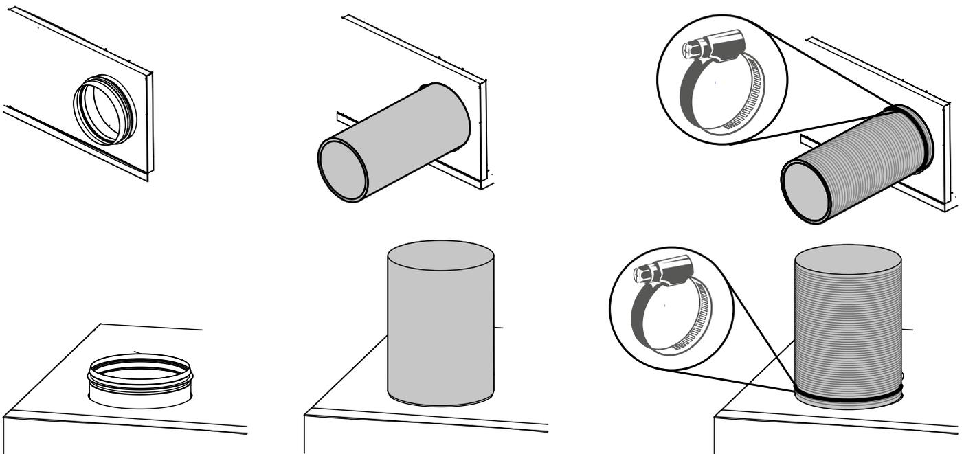
If the air ducts are too short or not connected, protect the unit parts from ingress of foreign objects.
