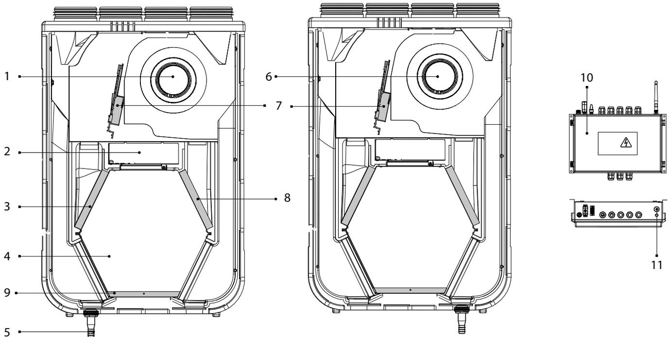
1 - exhaust fan; 2 - control unit (for VUT/VUE 270 V5(B) EC A2/A14 units); 3 - supply air filter; 4 - counter-flow heat exchanger; 5 - drain pipe (VUT 270 V5(B) EC); 6 - supply fan; 7 - bypass damper (only for VUT/VUE 270 V5B EC); 8 - extract air filter; 9 - drain pan; 10 - external control unit (for VUT/VUE 270 V5B EC A21 units); 11 - SETUP MODE button (for VUT/VUE 270 V5B EC A21 units).
