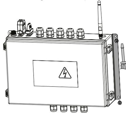
Design of hinges allows to change the opening side of a control unit cover. Unscrew the fixing screws, open the cover and unhinge it. Fix the cover to the opposite hinges, tighten the fixing screws.
