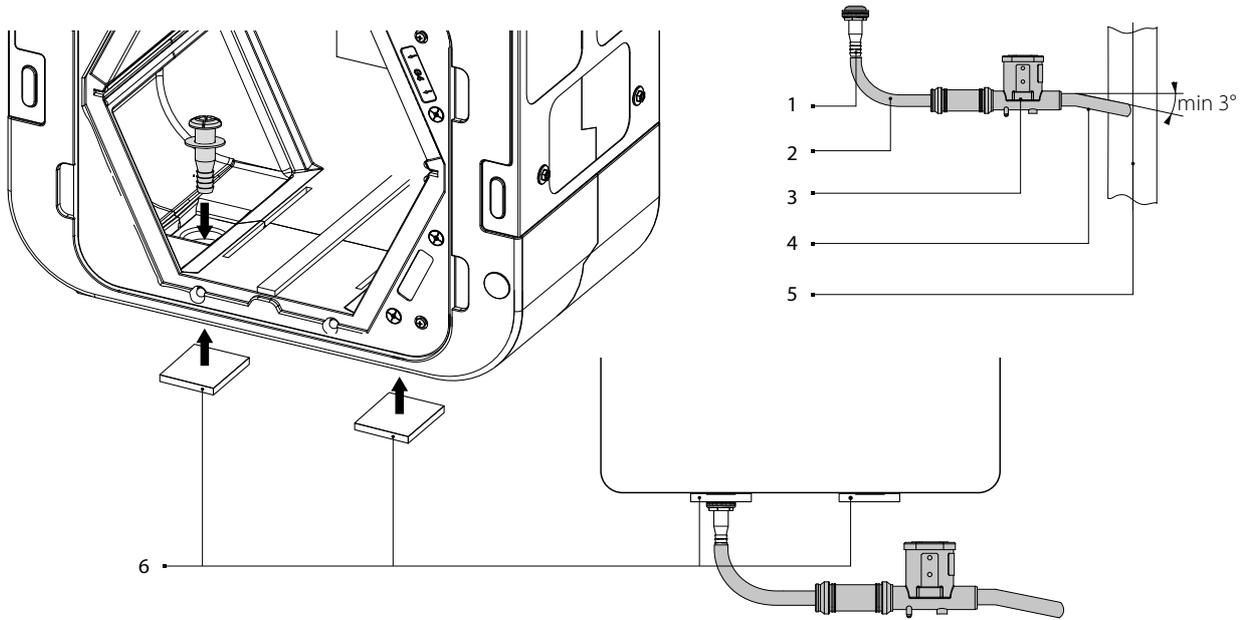
1 - drain pipe; 2, 4 - drain hose; 3 - U-trap; 5 - sewage system; 6 - additional insulation.
