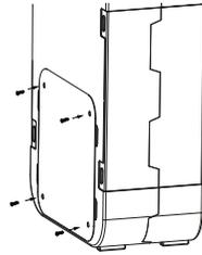
The plate opposite to the service side must be fixed with screws (included in the delivery set) before installation.
