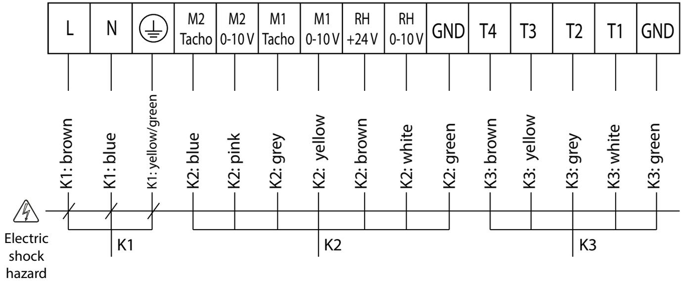
K1: Connection cable for M1, M2 motors and Y1, Y2 actuators.
